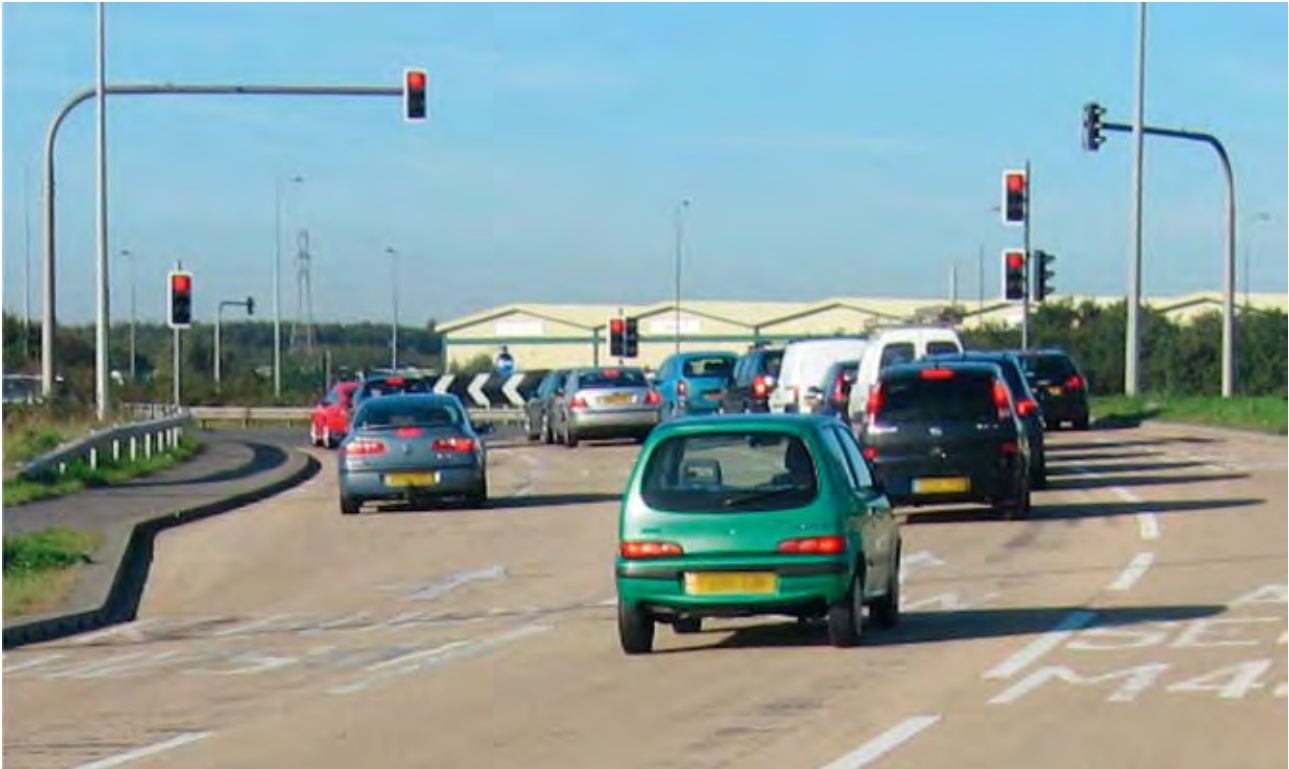
Figure 4.15 Mast arm signal – note location behind barrier
